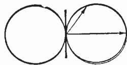
Fig. 102: Radiation from a dipole.
